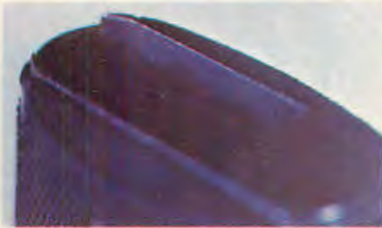
Above: Magazine well was beveled to author's specs for faster speed-loading of magazines under stress.
